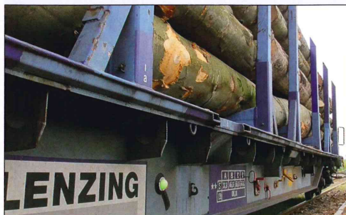
Overloading of wagons has thus become a thing of the past: The signal lamps immediately indicate up to seven loading situations. Transport companies benefit from achieving optimum load capacity, even with „difficult“ payloads such as wood, scrap and bulk consignments.
