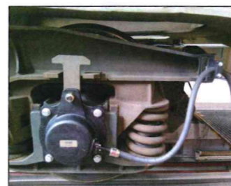
The WaggonTracker is energy self-sufficient, since the hub generator provides its power supply.
