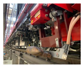
Impressive dimensions: 400 measurement channels and 30 telemetry channels collected data of 2 terabytes. PJM has a many years' experience of analysing such complex data.
