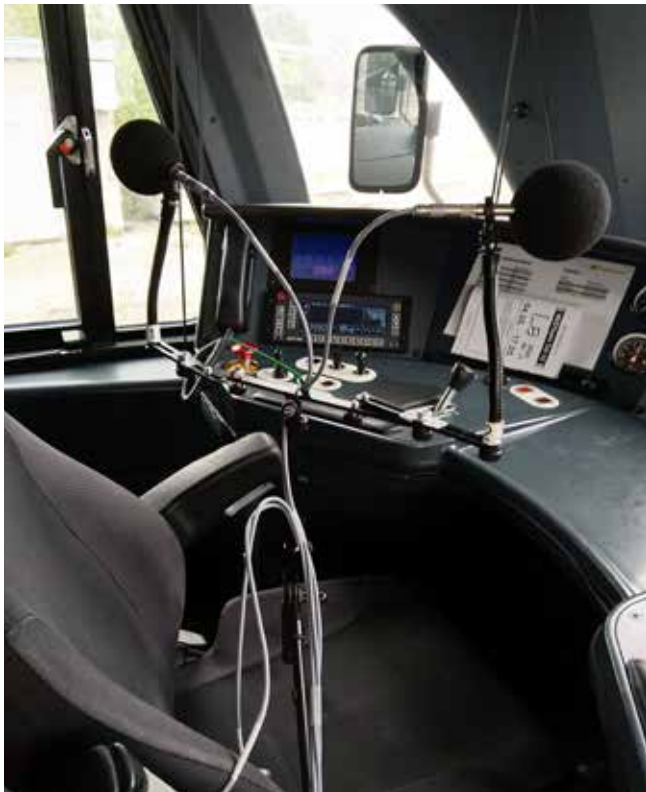
The acoustics were analysed according to TSI Noise 1304/2014/EU. Our PJM-experts determined stationary noise, starting noise and pass-by noise up to 200 km/h as well as driver's cab interior noise.
