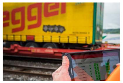
The new daily routine at SBB Cargo: Instead of the ergonomically unfavorable and strenuous manual control of the brakes, all results of the automatic brake test are displayed on the tablet.
