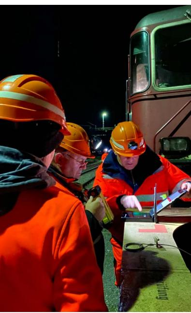
PJM's automated brake testing system has been evaluated and homologated by TÜV. The automated system has been undergone operational trials on more than 200 SBB Cargo freight cars.
