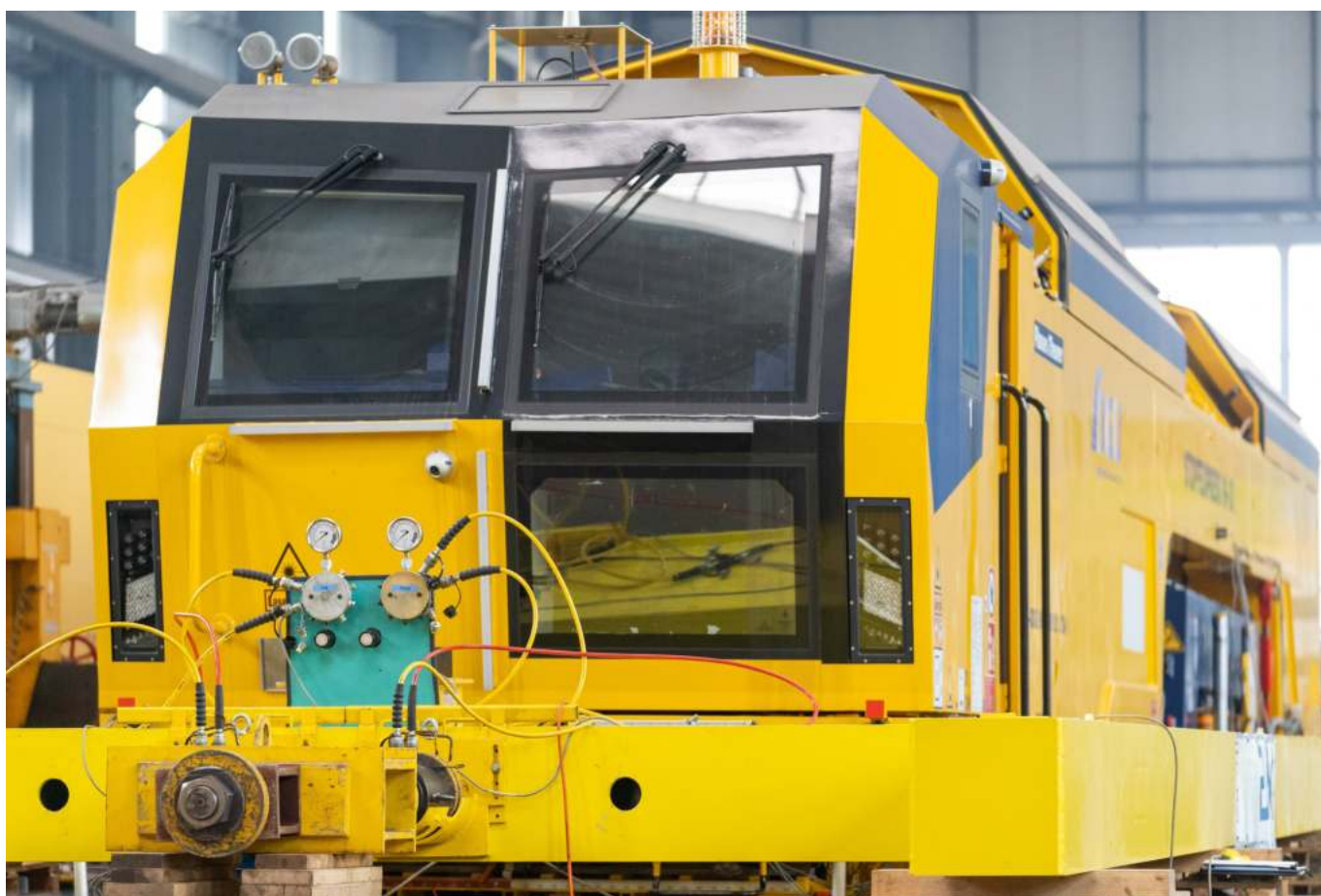
The mobile pressure frame is designed for every type of vehicle and thus also for special machines. Credit: Manuel Hanschitz, free of charge
