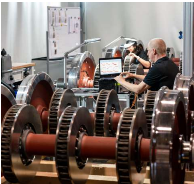
6 measuring wheel sets were developed and manufactured at the PJM site in Graz.
