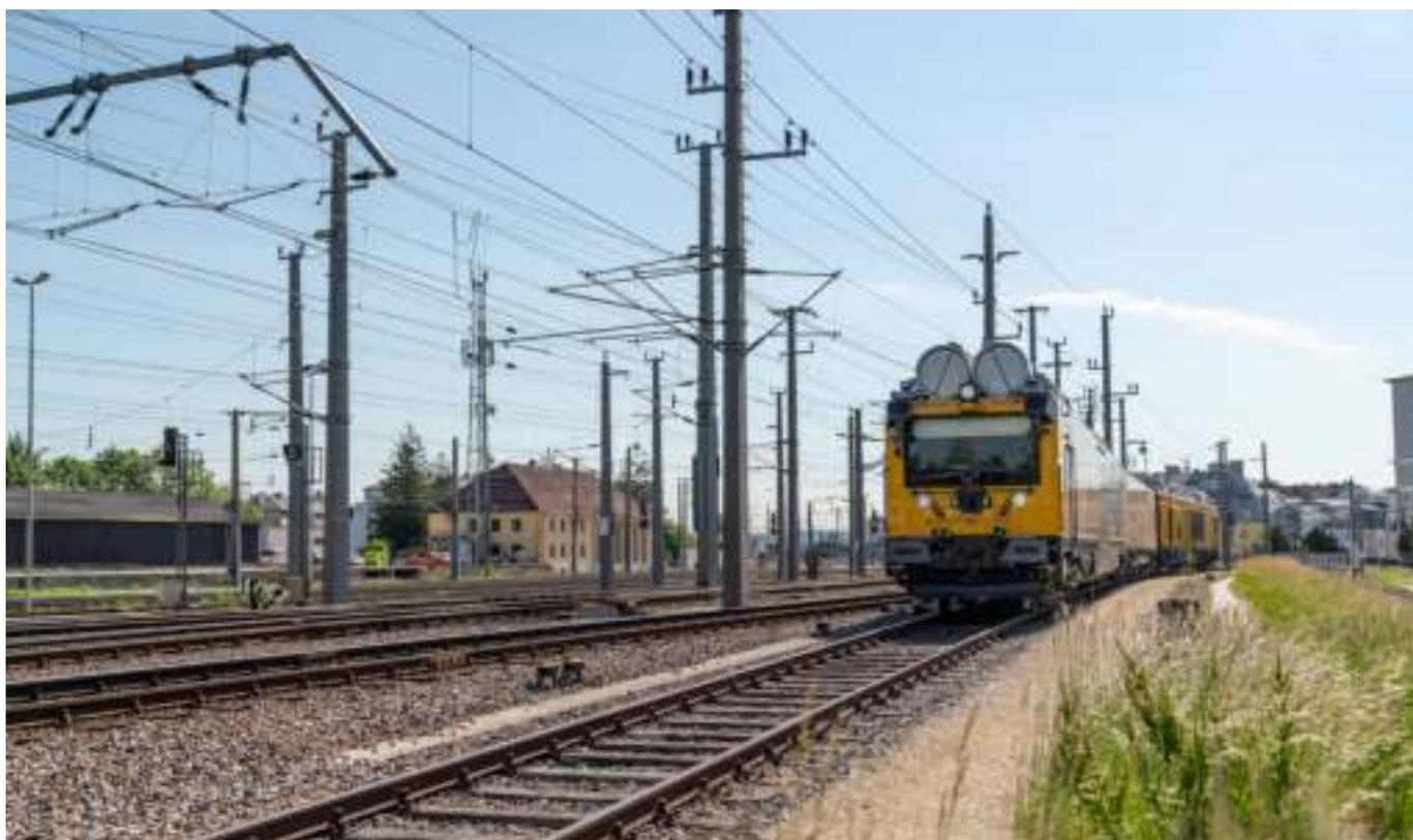
*The vehicle tests are carried out in the areas of running behavior, pantograph, acoustics and brakes.*
