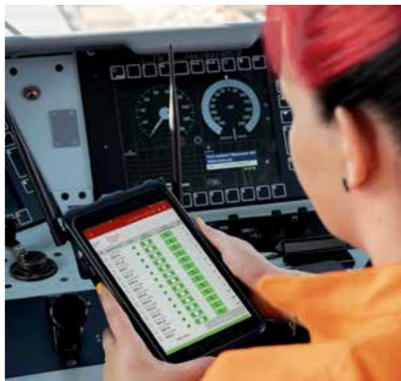
Above left: Swiss Federal Railways subsidiary SBB Cargo says it is the first operator to use the automatic brake test for freight trains. The approved process takes a few minutes and can be supervised by the driver of the train locomotive, reducing the need for shunting crews at terminals and marshalling yards.
