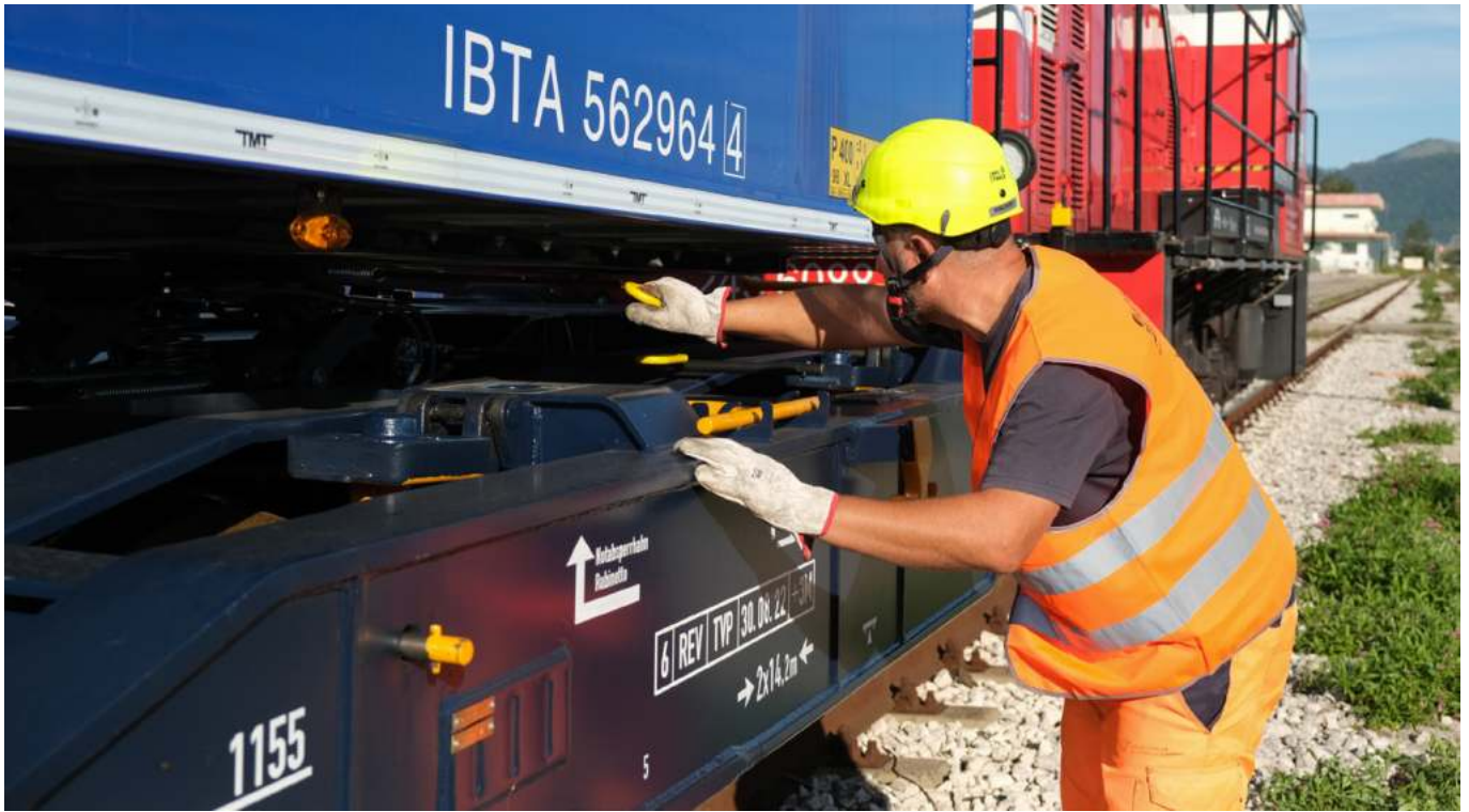
Real-time trestle monitoring enables reliable detection of the correct setting and locking during trailer transport in the intermodal sector Credit: Polo Logistica FS, free of charge
