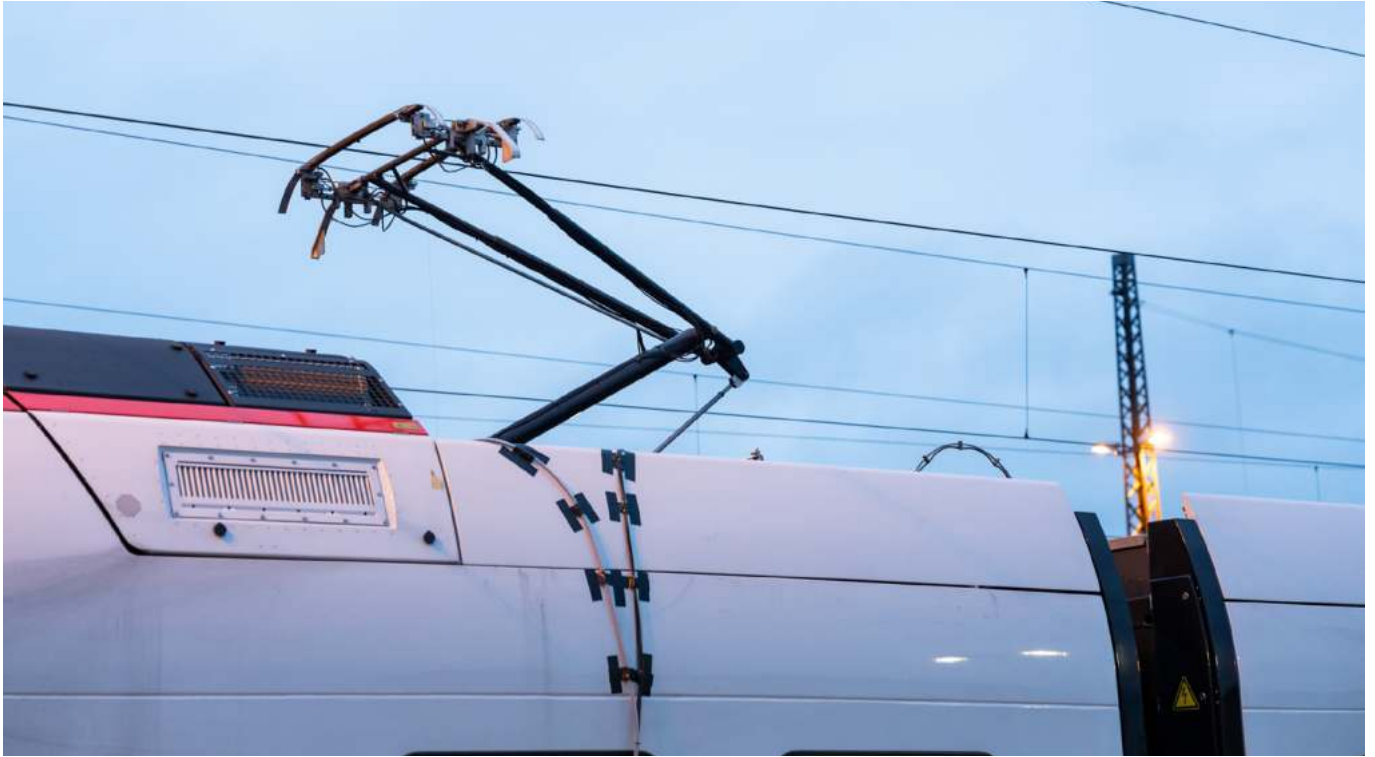
Synchronized recording of vehicle data and data from two measuring pantographs
