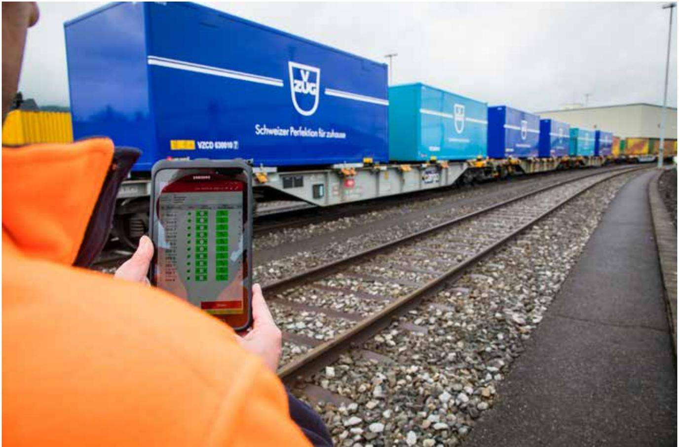
*For a 500-long freight train, the automated brake check takes less than 5 minutes. The automatic brake test fulfils all safety-relevant regulations in terms of operation and vehicle.*
