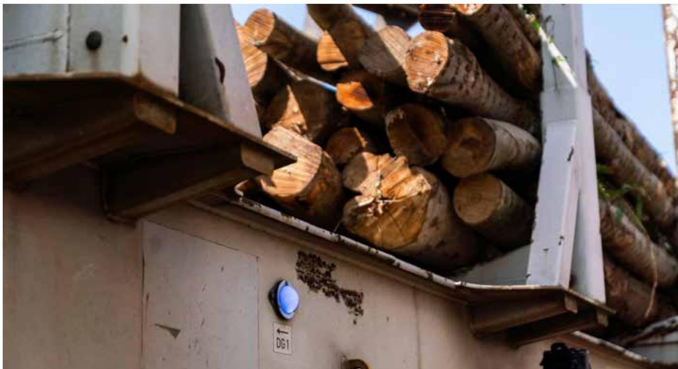
*On-site visualition in real-time via signal lamps. Automatic load weight monitoring indicates in real time during loading: Overloading, asymmetric loading, wheelset and wheel disc overloading, inadmissable load distribution on the bogie, loading level and loading is ok.*
