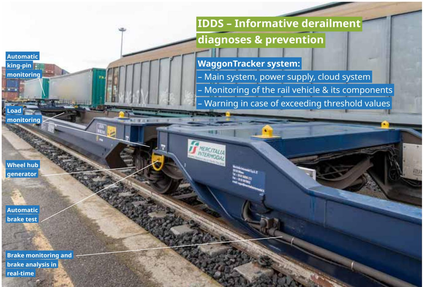
*The most intelligent freight train in Europe was realised for Mercitalia Intermodal. The extensive monitoring functions generate numerous advantages: shorter train preparation, faster delivery times, lower maintenance and repair costs, less wear on certain components, more efficiency and safety.*
