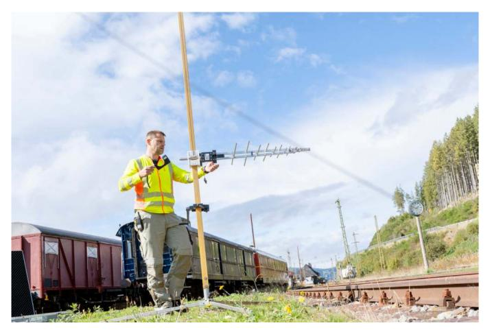
The newly founded EMC Rail Services GmbH offers EMC measurements in key areas such as radiated emissions, radio protection, personal protection and compatibility with track circuits, axle counters and other sensor-specific systems.
