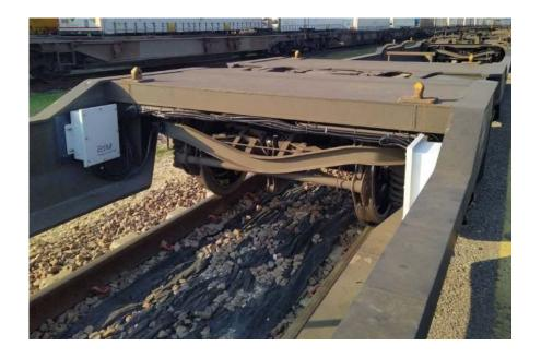
The WaggonTracker system of PJM serve sas the basic plattform for the "digital all-round equippment". Europe's most intelligent freight train by Mercitalia Intermodalia also features an automated brake testing system.
