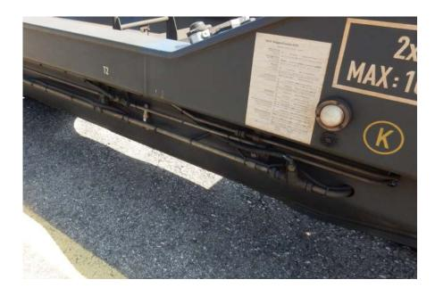
The loading status is also determined (load weight determination and its distribution) and is indicated during the loading process by signal lamps.
