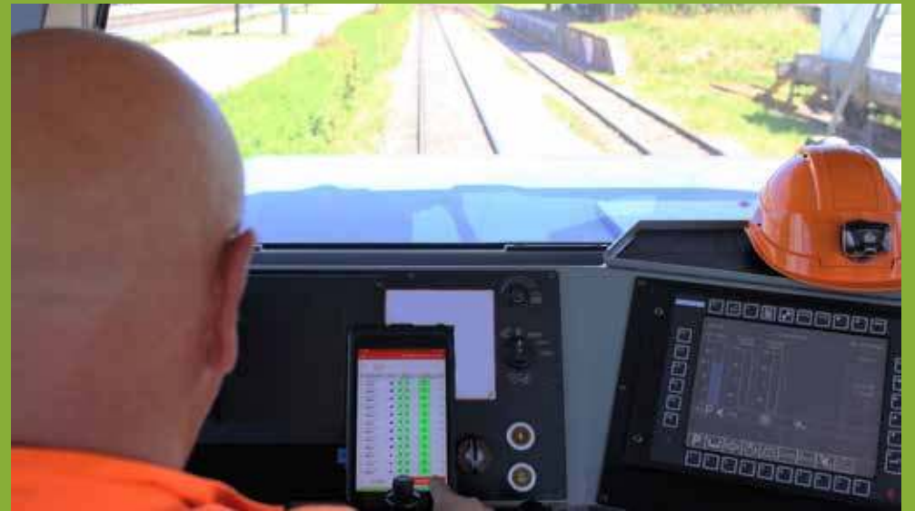
Everything in view with one click: The results of the automatically performed brake test are clearly displayed on the tablet of the train driver or brake test supervisor.
