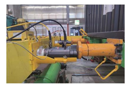
For the static strength test according to EN 12663, the mobile pressure frame was used, which is an in-house development by PJM. The vehicle frame is subjected to different loads in order to determine the distortions and stresses that occur.
