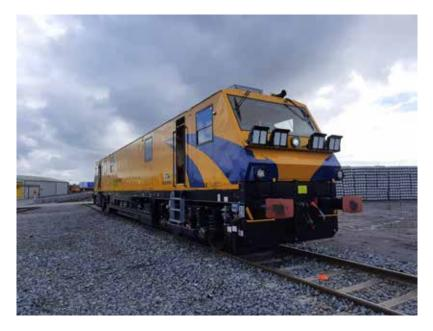
ISO/IEC 17025 accredited systems specialist PJM conducted the testing of two rail inspection vehicles for Geismar Italia S.p.A in the areas of running behavior, brakes and acoustics in Ireland.
