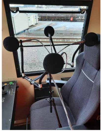
PJ Messtechnik GmbH /// Waagner-Biro-Straße 125, 8020 Graz, Austria T: +43 316 22 84 54 /// E: office@pjm.co.at /// **www.pjm.co.at**  Acoustic measurements according to TSI NOI 2014/1204/EU were used to investigate pass-by noise, rail roughness and decay rate. Acoustic measurements according to TSI NOI 2014/1204/EU were used to investigate pass-by noise, rail roughness and decay rate.
