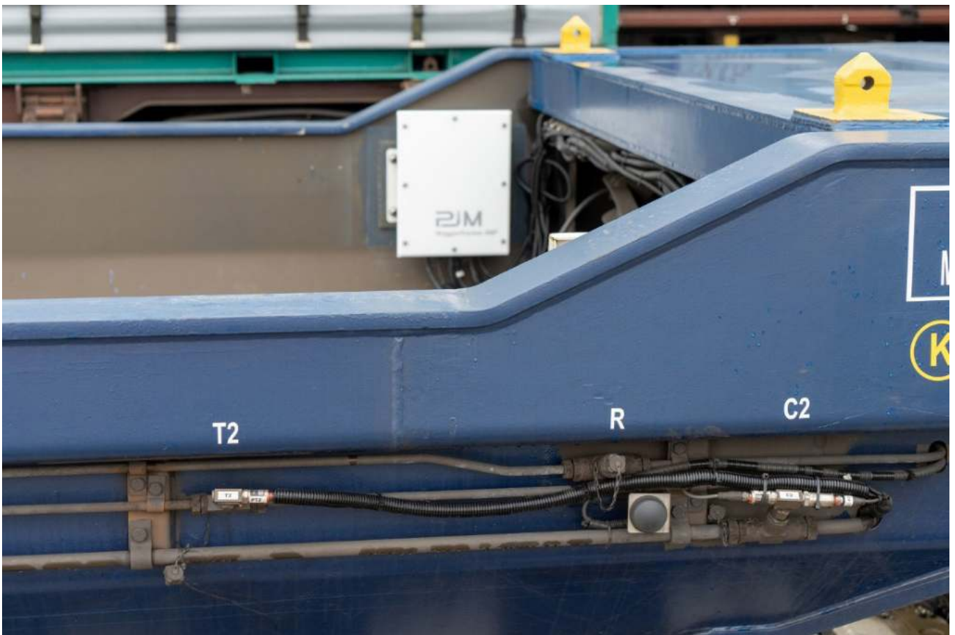
Mercitalia Intermodal benefits from numerous monitoring features, among many the real-time brake analysis and brake system monitoring while travelling and at a standstill. Credit: PJM, free of charge
