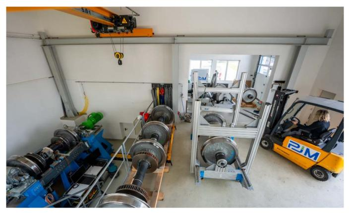
The infrastructure in the field of instrumented wheelsets includes a stationary test rig, a dynamic test rig and the corresponding technical equipment such as an indoor crane.
